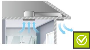
Blauberg fans comply with the Building Code requirements of Thermal Performance, by including a backdraft damper in the majority of our fans. This is designed to seal off the fan when not in use. Backdraft dampers are available as an accessory for code compliance.
