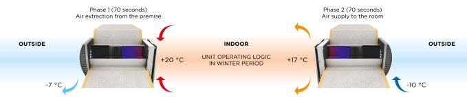
Warm stale air is extracted from the premise, flows through the ceramic heat exchanger and transfers its heat and moisture to it.
