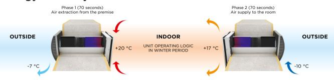
Warm stale air is extracted from the premise, flows through the ceramic regenerator and transfers its heat energy and moisture to it.
